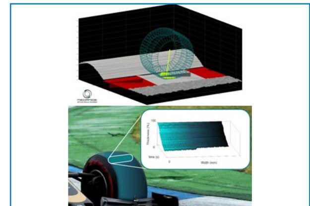
Virtualization of a motorsport tire for real-time simulations and the prediction of grip and wear performances
