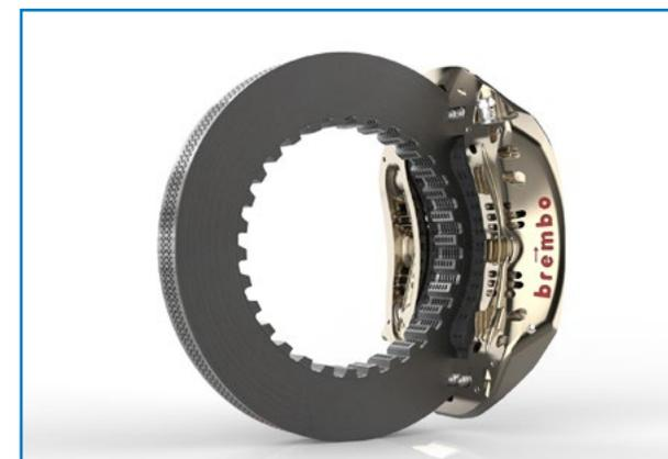
Braking system for the Formula 1 Championship: carbon disc, carbon pads, six-piston lithium-aluminum monobloc caliper
